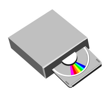
CD-ROM stands for Compact Disk-Read Only Memory. They are flat, shiny disks that sto information. Most new computers have CD-RW drive CD-RW stands for Compact Disk-ReWrite. This type of disk allows you to write information to it, as well as read from it. Most can hold up to 700 megabytes of information.
