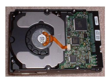
Hard Disk Drives use Magnetic Recording Techniques. The magne medium can be easily erased and rewritten an will "remember" the magnetic flux patterns stored on it for many years!
