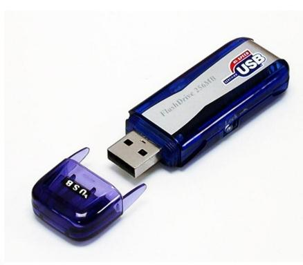
A Flash Drive is a relatively new storag device. It's like a mi portable hard drive! You plug it into the USB (Universal Serie Bus) port on the from of newer computers and you can save to it!
